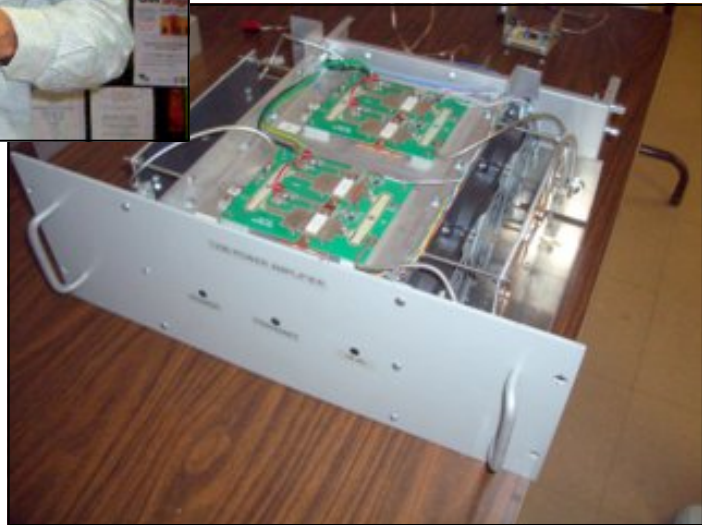
An example of Phil's very fine workmanship on his 1296 MHz SSPA
